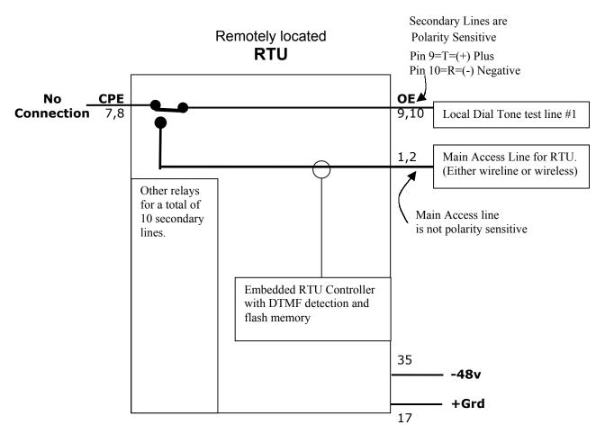
See Application Note-24 for attaching multiple RTUs for more than 10 secondary lines.
